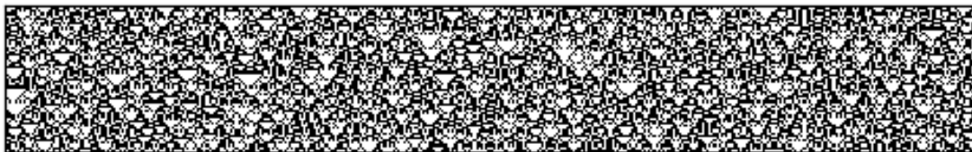
Figure 1: Space-time diagram of Rule 90; with local rule f(x, y, z) = (x + z) \bmod 2 ; operating on a cyclic configuration of size 250. Time flows downwards.
