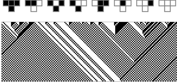
Figure 2: Rule 184 rule table and space-time diagram.
